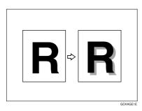
This function adds a shadow around the edges of copy image elements. You can select block shadow or offset shadow.
